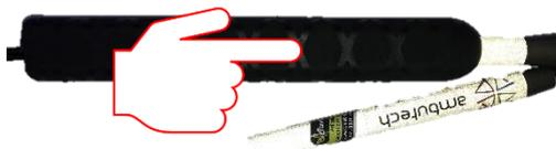
Each cane in close proximity will detect the presence of the TAG in ASSOCIATION mode. Press the P2 button of the cane twice to confirm the pairing.
