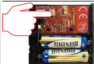
When the TAG is ON, press the button in the compartment; a sound signal will be activated to indicate the activation of the ASSOCIATION mode.
