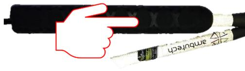
Each cane in close proximity will detect the presence of the TAG in ASSOCIATION mode. Press the P2 button of the cane twice to confirm the pairing.
