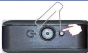
When the TAG is ON, **press the button in the compartment**; a sound signal will be activated to indicate the activation of the ASSOCIATION mode.
